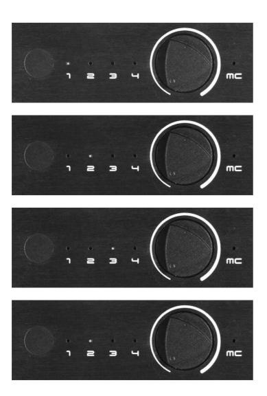
If you turn on the CIA-1 in the standby mode, the last selected channel selection in the EEPROM is stored. After restarting the device starts with the last channel setting.
