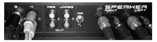
With the switch between unregulated RCA output and the speaker output sockets you can switch the CIA-1 into the pure Power Amplifier mode. Input 2 is switched active. The volume control is bypassed.
